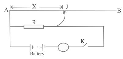
You are provided with a potentiometer **AB**, a  $10\Omega$  standard resistor **R**, a battery of *emf* 4.5, a jockey **J** and other necessary materials.
