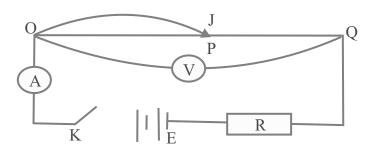
You are provided with a potentiometer, an ammeter, a voltmeter, standard resistor and other necessary apparatus. Using the circuit diagram above as a guide, carry out the following instructions.
