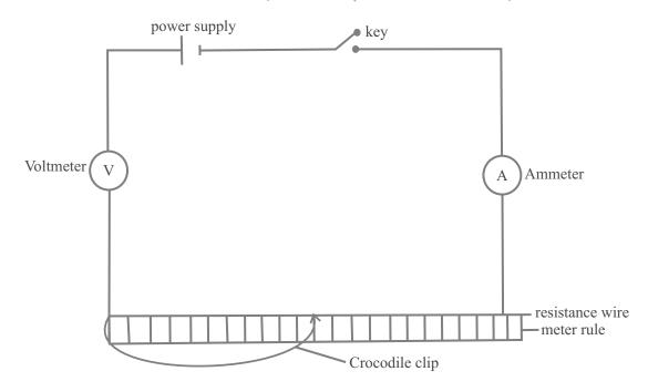
In this experiment, you will investigate how the resistance of a length of wire depends on its diameter.
