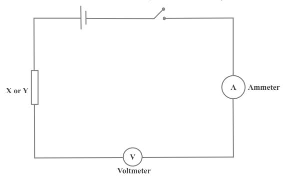
In this experiment you will make some measurements on an electrical circuit that contains various combinations of resistors.
