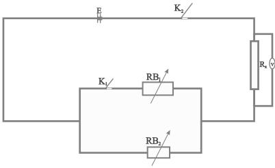
You have been provided with an accumulator E, a standard resistor Rx, two resistance boxes RB1 and RB2 two keys k1 and k2 and other necessary apparatus.
