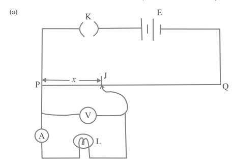
You are provided with cells, a potentiometer, an ammeter, a voltmeter, a bulb, a key, a jockey and other necessary materials.
