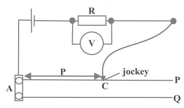
The circuit shown above is set up to investigate how the potential difference across the fixed resistor R varies when extra resistance is included in the circuit. The extra resistance is obtained from different lengths of two resistance wires P and Q. From the results, the resistance of the two wires is to be compared.
