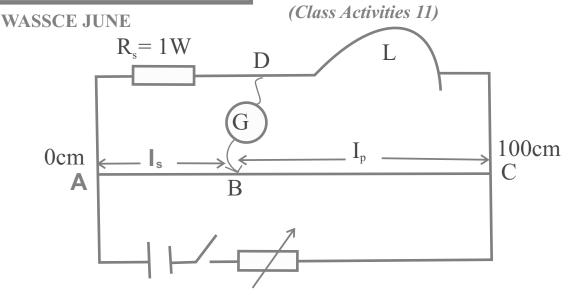
You are provided with two wires marked P and Q, a resistor  $R_s = 1\Omega$  and other necessary apparatus.
