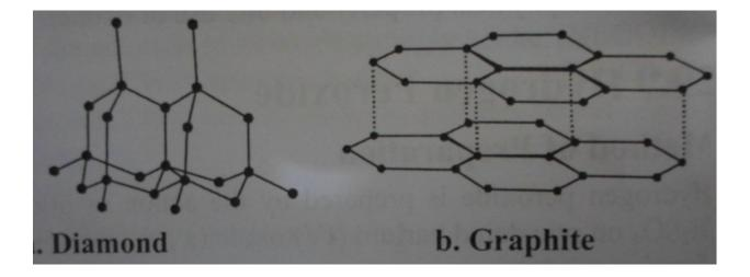
The rigidity of the structure is responsible for the hardness of diamond; it is the hardest known substance. Since the covalent bonds are strong and the molecule is compact, the melting point of diamond is very high.
